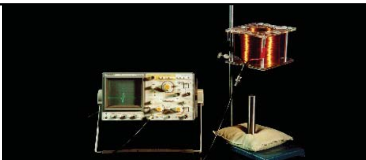
Motional induction demonstration: The magnet is dropped through the coil of wire, and the resulting induced emf is displayed on the oscilloscope.
