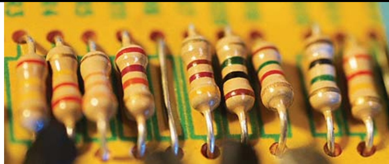
Resistors wired into a computer circuit board. Each resistor has a color code that indicates its resistance in ohms.
