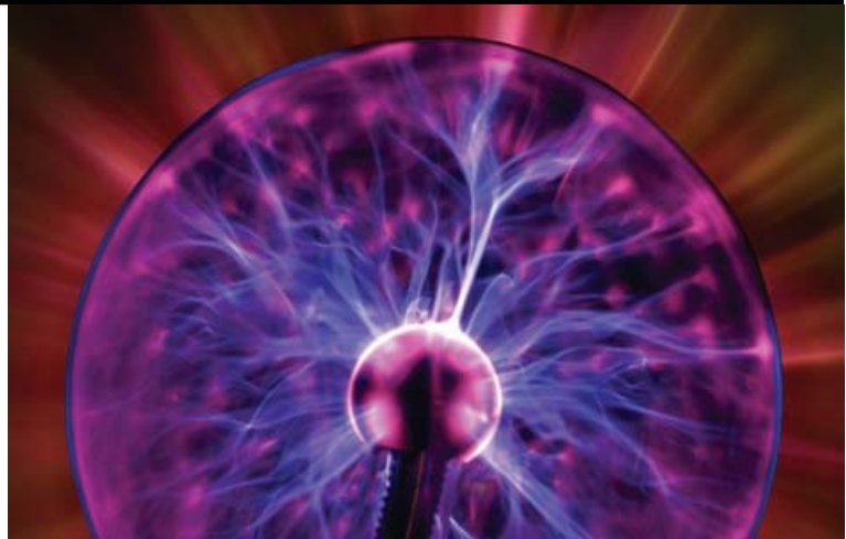
Charge resides on the surface of the inner metallic sphere in this toy. An electric field extends radially outward, made visible by ionized gas.
