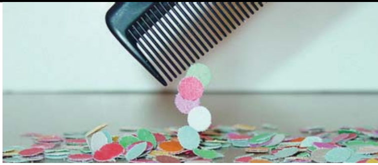
A charged comb induces electric charges in the paper dots which cause them to stick together. This phenomenon is called static cling.
