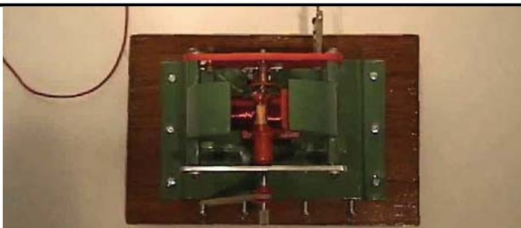
DC electric motor. The sparking copper commutator is visible between the rotors and the red plate at the top of the image.
