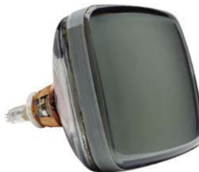
TV tube. A gun (far left) accelerates electrons across a potential difference. Electromagnets (brown) steer the moving charges to light up screen pixels.
