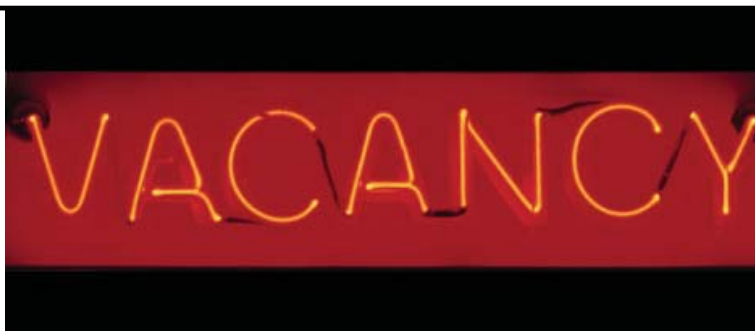
The electrically excited neon gas in this sign emits light at several sharply defined red-orange wavelengths.
