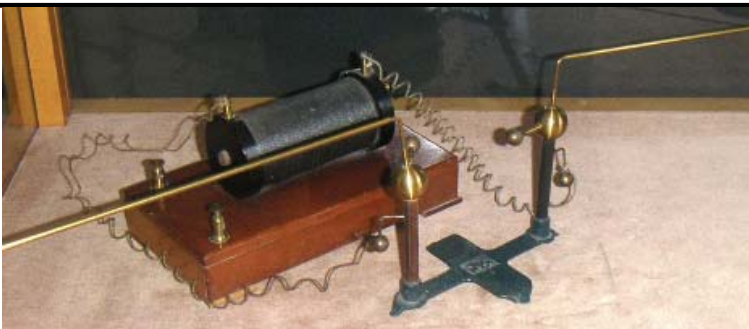
Heinrich Hertz transmitter, 1888. Transformer voltage causes a spark to jump between the positionable brass spheres, generating a radio pulse.
