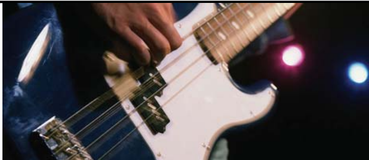
The pickups (raised black modules) on this electric guitar convert the vibrations of the strings into a varying electric current.
