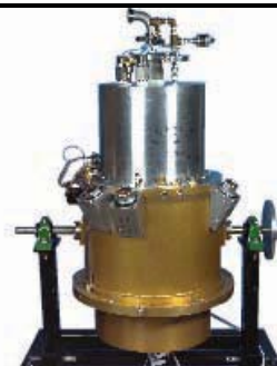
This advanced flywheel is being developed by NASA as a source of stored energy for use by satellites and spacecraft.
