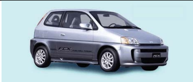
This Honda FCX automobile can cruise up to 350 km by using the electric potential energy stored in its capacitors as a configuration of electric charge.
