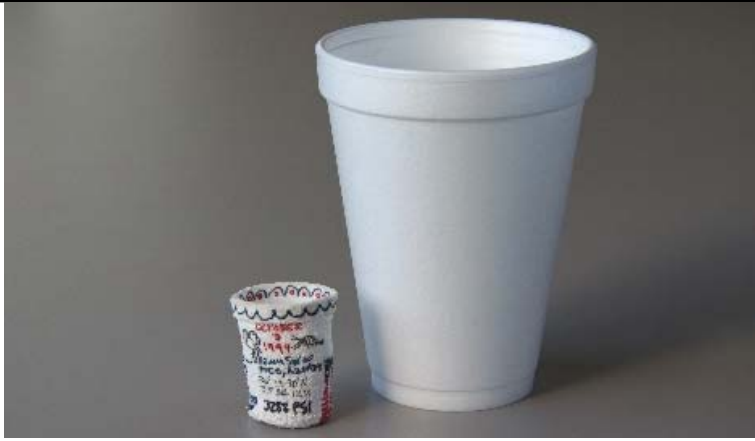
The effect of volume stress on a Styrofoam cup submerged 7875 feet underwater (with an un-stressed cup also shown for comparison). The stress on the cup exceeded its elastic limit: it is permanently deformed.
