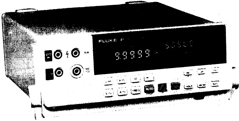
Figure 15-9 Fluke 45 dual display multimeter which can make two measurements on one input signal. (© 1988, 1990, John Fluke Mfg. Co., Inc. All rights reserved. Reproduced with permission.)
