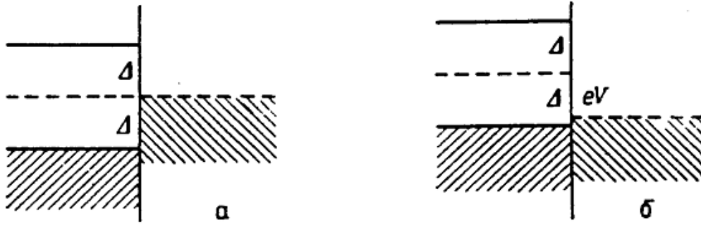
Figure 20.4: Energy diagram for N-S tunneling (S – left side, N – right side of each panel).
