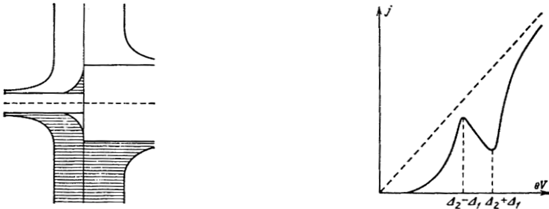
Figure 20.5: S-S tunnelling. Left – Energy diagram, right – I - V -curve.
