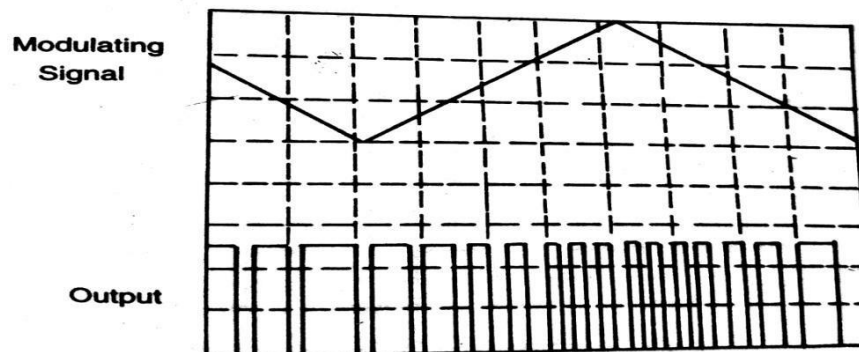
Fig. 8.23 Pulse position modulator output
