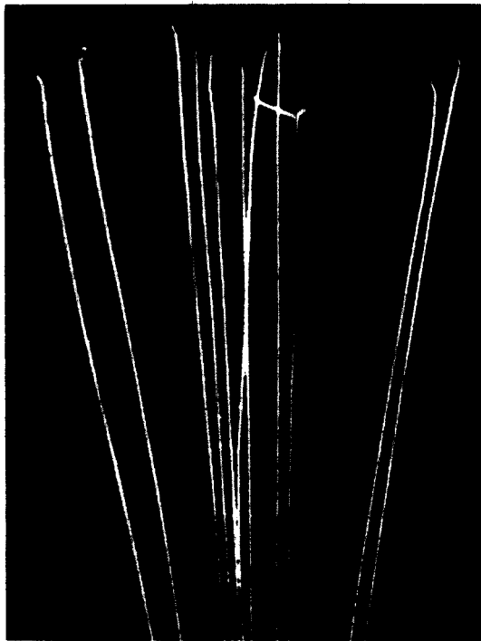
FIG. 13-4. A cloud chamber photograph showing the straggling of \alpha -particles from Thorium C'. The last three centimeters of range are shown. [Reprinted by permission from Rutherford, Chadwick, and Ellis, Radiations from Radioactive Substances . New York: Macmillan, 1930.]
