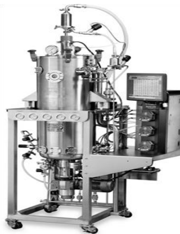
Figure 3 Stainless Steel Fully Automatic 10-dm 3 Fermenter Sterilizable-In-Situ (LSL, Luton, UK)
