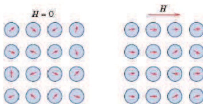
Figure 2: Atomic dipole configuration for a paramagnetic material without and with magnetic field.
