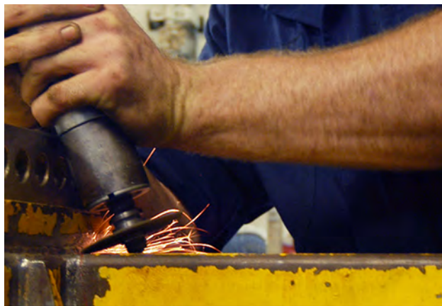
Figure 8.6 A grinding wheel applies a non-conservative force, because the work done depends on how many rotations the wheel makes, so it is path-dependent. (credit: modification of work by Grantez Stephens, U.S. Navy)
