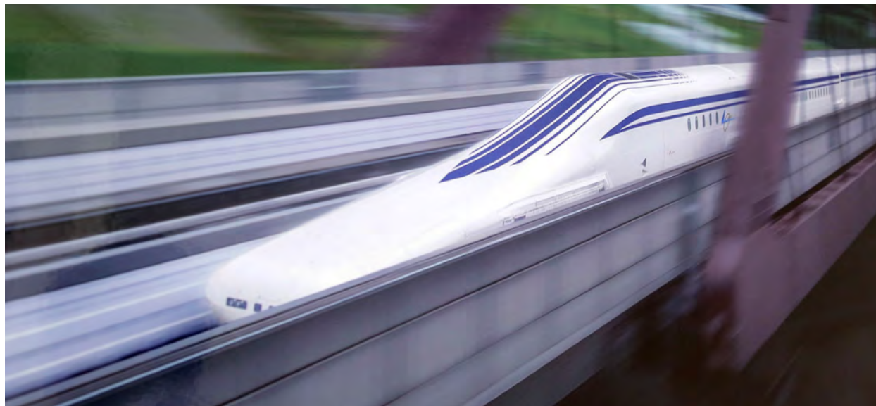
Figure 3.1 A JR Central L0 series five-car maglev (magnetic levitation) train undergoing a test run on the Yamanashi Test Track. The maglev train’s motion can be described using kinematics, the subject of this chapter. (credit: modification of work by “Maryland GovPics”/Flickr)
