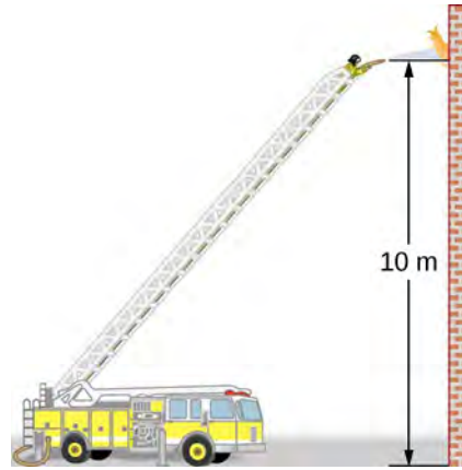
Figure 14.33 Pressure in the nozzle of this fire hose is less than at ground level for two reasons: The water has to go uphill to get to the nozzle, and speed increases in the nozzle. In spite of its lowered pressure, the water can exert a large force on anything it strikes by virtue of its kinetic energy. Pressure in the water stream becomes equal to atmospheric pressure once it emerges into the air.
