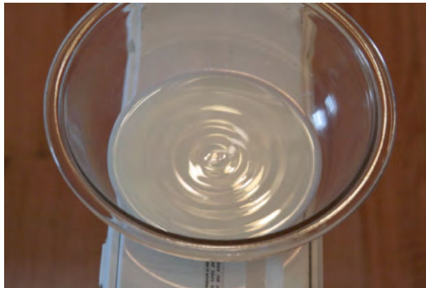
Figure 16.25 Standing waves are formed on the surface of a bowl of milk sitting on a box fan. The vibrations from the fan causes the surface of the milk of oscillate. The waves are visible due to the reflection of light from a lamp. (credit: David Chelton)
