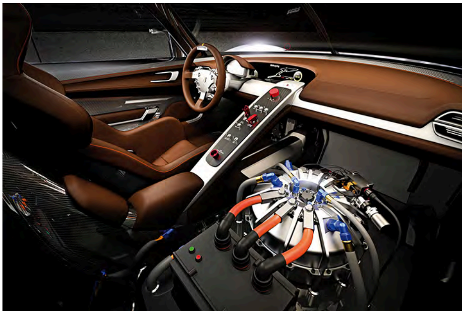
Figure 10.18 A KERS (kinetic energy recovery system) flywheel used in cars. (credit: “cmonville”/Flickr)
