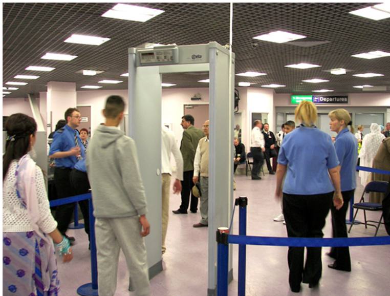
Figure 14.9 The familiar security gate at an airport not only detects metals, but can also indicate their approximate height above the floor. (credit: “Alexbuidrs”/Wikimedia Commons)
