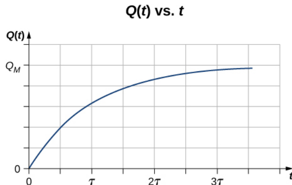
Figure 9.3 A graph of the charge moving through a cross-section of a wire over time.
